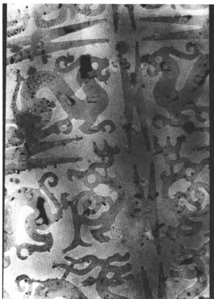
Figure 12. X-ray radiograph of section of the wall of the Hu shown in Figure 11. From the evidence seen in this radiograph—square and rectangular supports behind each figure, the white spots on or near each rod (solder), and dark areas (voids in metal) around each figure—the casting procedure described in the text can be deduced. Exposure: 275 kV, 4 mA, lead screens.
