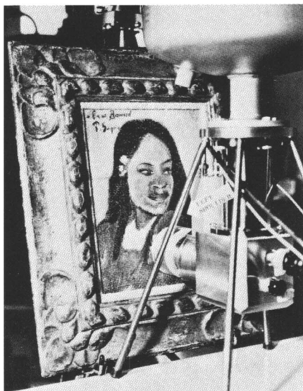
Figure 1. X-Ray fluorescence analysis of a painting (90)
