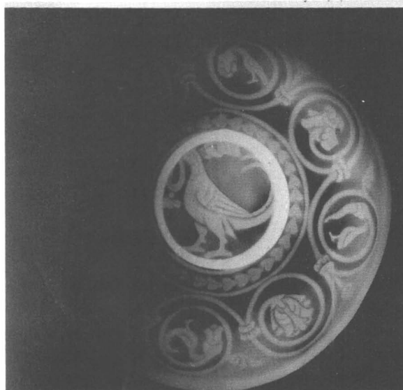
Figure 7. (top) Sasanian silver gilt plate, The State Hermitage Museum, Leningrad, U.S.S.R. Figure 8. (bottom) X-ray radiograph of Sasanian silver plate shown in Figure 7. Decorated sections appear as lighter areas indicating solid metal. This radiograph is typical for hammered Sasanian silver plates with a carved relief decoration; the light circle in the center is the radiographic impression of the foot ring. Radiograph obtained with Philips PG 200 x-ray unit, 200 kV, 3 mA, no screens.
